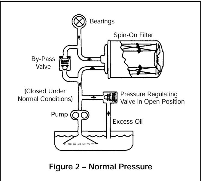
Automotive lube oil filters are designed to withstand differential pressures significantly greater than those experienced under normal operating conditions without collapsing. Therefore, when an element has collapsed, it is usually the result of a "sticky" or otherwise malfunctioning by-pass valve.
