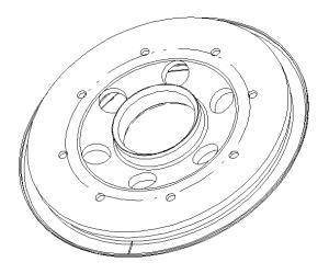
Also, the hole pattern was changed from 8 to 6. Fewer holes provide additional strength to the assembly as well.
